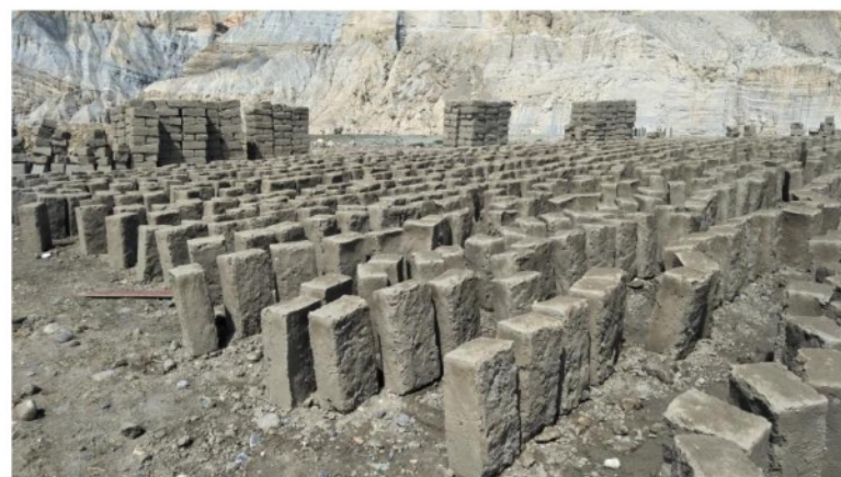
Clay Mud Brick for house wall construction
